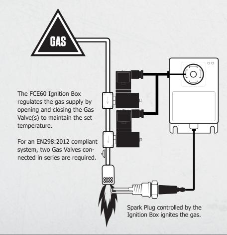
The FCE60 Ignition Box controls ignition of the flame and monitors it. Upon ignition failure, it closes the gas valve as a safety measure to prevent accidents caused by gas seepage and presents an error code.
