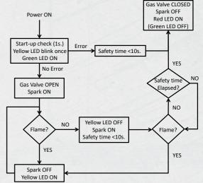
When power is applied the Ignition Box opens the gas supply and starts igniting (after a brief start-up check). If the Ignition Box detects a flame, the yellow lamp will turn on and the Ignition Box will cease sparking. After this, the Ignition Box will continue to monitor the flame, and as long as the flame is detected, the yellow lamp stays on.
